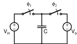
$$E_{loss} = C(V_{max} - V_{min})^2$$
